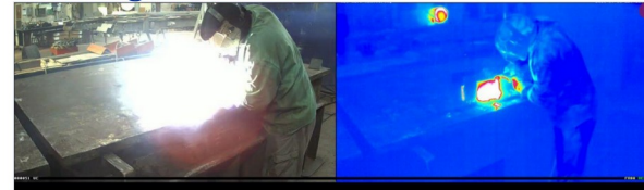
Same instant, two views — standard camera (left) vs. thermal (right). The heat signature is visible before any flame is.
